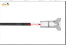
If the injector steel ball and the ball seat are not installed in accordance with the standard, it may cause serious damage to the injector valve assembly.
