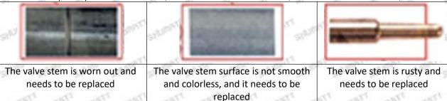
The excessive clearance between the stem wear and the housing and between the cap causes an injector delay
